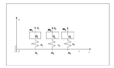
The computational scheme for the system represented by the console rod with three oscillators presuming damping
