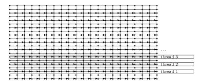
Fig. 3. Matrix element traversal order and its distribution into threads
